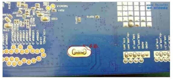
Step 2: Find a few key pin test points DO,CMD,CLK,GND,at least 4 lines,and the line should be better within 10cm.
