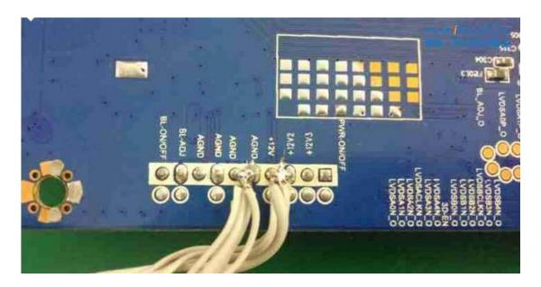
Step 4: Supply the 12V power to the Liquid Crystal mainboard, open the software of the programmer, choose EMMC\_AUTO\_ISP and then click "Read".
