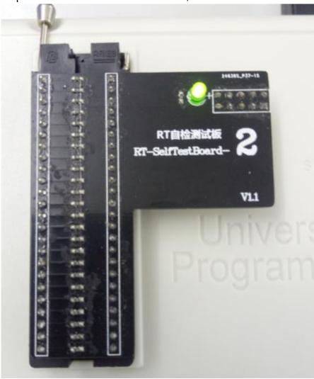
Step 6 : Click ,check the hint in the software,it will hint "Selftest 2, test pass" ;
