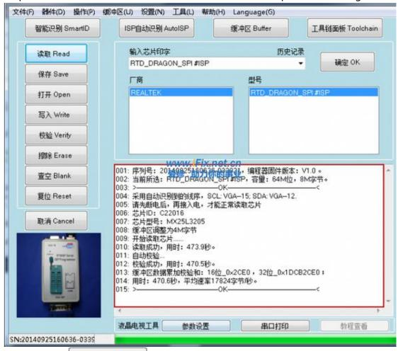
Step 4 : Click to save the file after finishing reading. Try the best to name the file in detail, including the manufacturer, board number, screen type, main chip type, memorizer type for the convenient use in the later.
