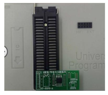
Use the putting position of simple switch board,,when welding chip the 1 foot is at the lower left.(Support the 93XX,24XX,25XX to be placed at will)
